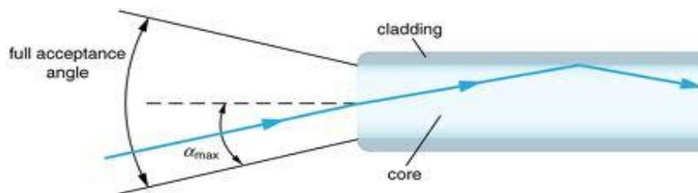
**Light Propagation through optical fiber**
