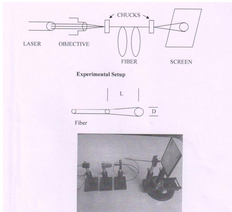
**Fig. 1:** Experimental setup for NA measurements
